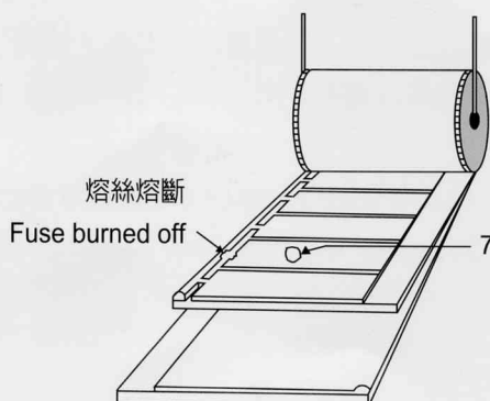
Figure 2. Fuse burned off on failure area
